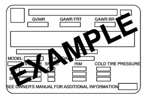
A vehicle specific Certification/Tire label is attached to the lower area of the center pillar (B-pillar). The label shows the gross weight capacity of your vehicle. This is called the Gross Vehicle Weight Rating (GVWR). The GVWR includes the weight of the vehicle, all occupants, fuel, cargo, and trailer tongue weight, if your vehicle is pulling a trailer.
